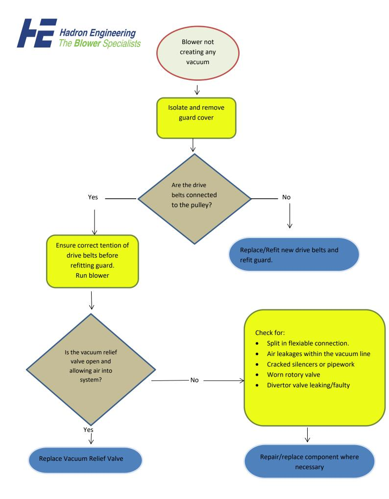
NOTE – A blower is an air mover it moves air from the inlet to discharge the blower itself does not create any vacuum it is the restrictions within the system pipework and the system that creates the vacuum.
