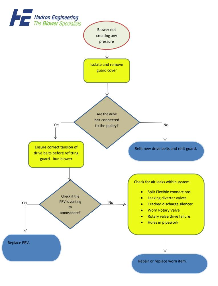
NOTE – A blower is an air mover it moves air from the inlet to discharge the blower itself does not create any pressure it is the restrictions within the system pipework and the system that creates the pressure.
